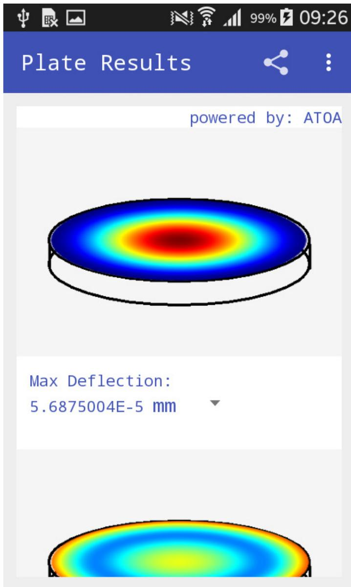
\* The results window will display the plate, deflection, stress and along with material, load, and boundary and analysis details.
